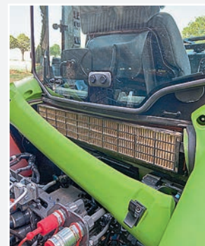
The filter is difficult to access with an implement attached.
