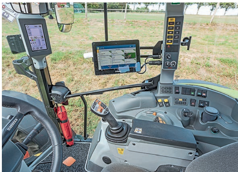
The joystick is also a cross control – ideal for loader work.
