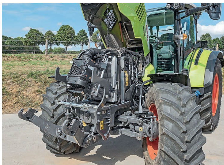
The four-cylinder FPT motor is quiet and very economical. Photos: Stefan Tovornik, Hubert Wilmer.
